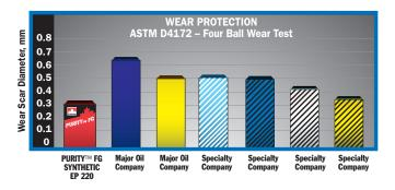
PURITY FG SYNTHETIC EP Gear Fluids deliver stronger wear protection than many major oil companies' and specialty lubricant suppliers' fluids. Less wear means fewer production upsets, higher productivity and helps to lower maintenance costs.
